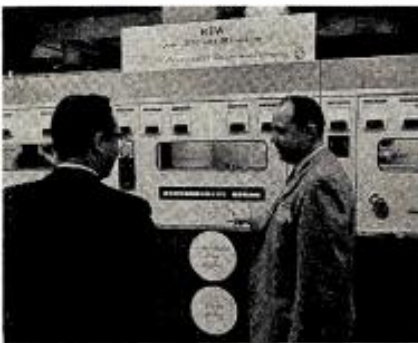
Vernon Collins (r) of LTV Continental Electronics Division stops a prospect with easy control feature of firm's new 50-kw AM transmitter.
