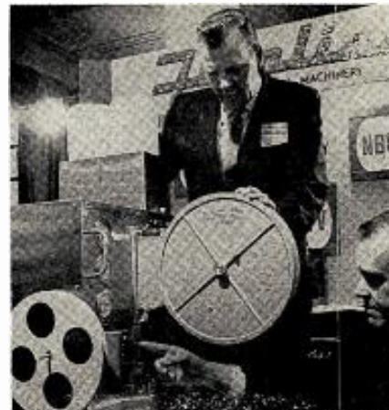
Jack Grady (r) and Herb Swenson of Filmline Corp. show firm's portable film processor, which can handle up to 70 feet per minute negative film.
